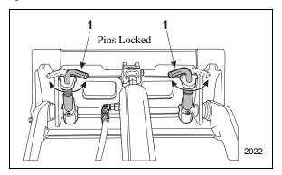
Figure 3-28 Attachment Locks in Locked Position
